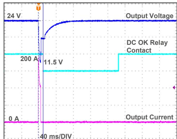
Fig. 8.4 APB 500% of nominal output current for 5 ms
