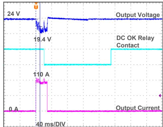
Fig. 8.2 APB 275% of nominal output current for 25 ms
