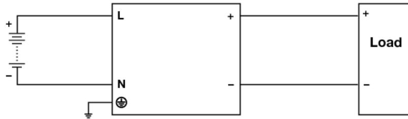
Fig. 6 DC Input Operation Connection Diagram
