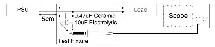
Fig. 3 Ripple & Noise measurement circuit
