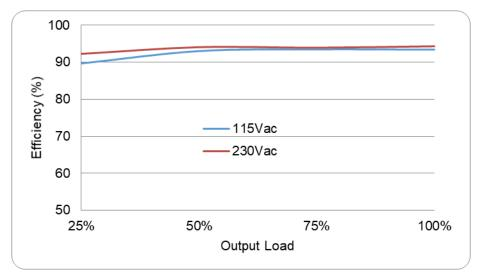
Fig. 1 Efficiency versus output load
