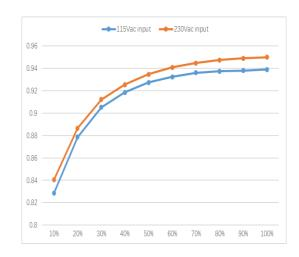
Figure 1-1. Typical efficiency Curve for 48V (600W max)
