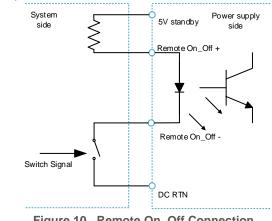
Figure 10. Remote On\_Off Connection
