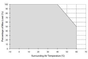
Fig.1.1 De-rating for Mounting Orientation A to F > 50°C de-rate power by 2.5% / °C
