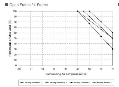
Fig.1.1 De-rating for Mounting Orientation A, C > 50°C de-rate power by 2% / °C De-rating for Mounting Orientation B, E > 45°C de-rate power by 2% / °C De-rating for Mounting Orientation D > 40°C de-rate power by 2.33% / °C De-rating for Mounting Orientation F > 40°C de-rate power by 1.66% / °C
