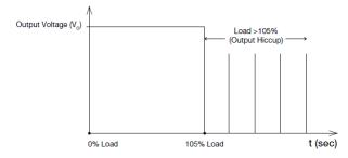
Additionally, if the I<sub>0</sub> is <105% but >100% for a prolong period of time (depending on the load), the Over Temperature Protection (OTP) will be activated due to high temperature on critical components. The power supply will then go into latch mode until the fault is removed and the mains is reapplied.
