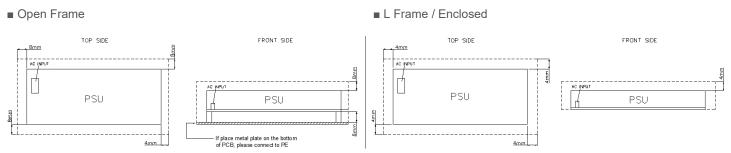
For safety reasons, please ensure the mounted device is kept safety distance as below at all sides from other components and equipments. a) For Open Frame Type  $\ge 8 \text{ mm} (0.315 \text{ inch})$  from primary side and  $\ge 4 \text{ mm} (0.16 \text{ inch})$  from secondary side.
