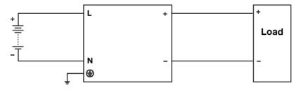
Fig. 4 DC Input Operation Connection Diagram
