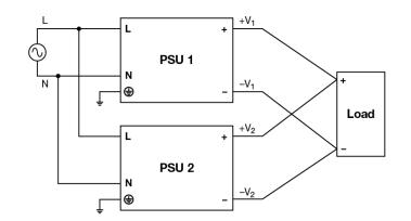
Fig. 3 Parallel Operation Connection Diagram
