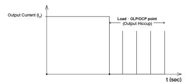
It is not recommended to prolong the duration of  $\rm I_{0}$  when it is less than OLP/OCP point, but greater than 100%, since it may cause damage to the PSU.
