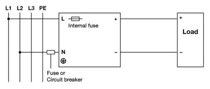
Fig. 5 2 of 3 Phase System Input Operation Connection Diagram
