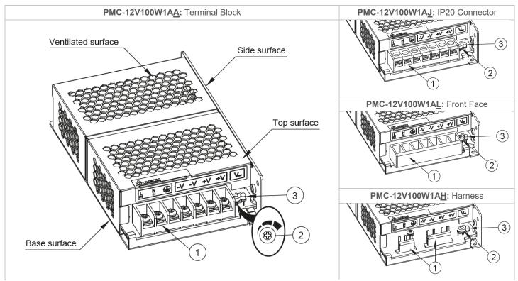
1) Input & Output terminal block connector
