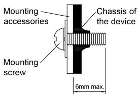
Only use M3 screw ≤ 6 mm (0.24 inch) through the base mounting holes. This is to keep a safety distance between the screw and internal components.
