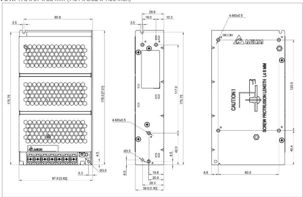
■ PMC-12V150W1B<u>J</u>: IP20 Connector L x W x H: 178 x 97 x 38 mm (7.01 x 3.82 x 1.50 inch)
