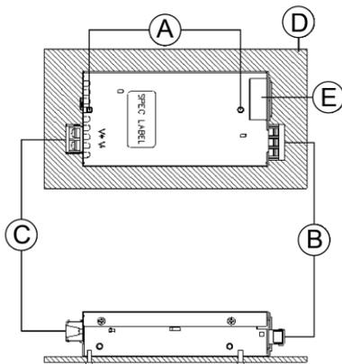
Fig. 2 Mounting Orientation
