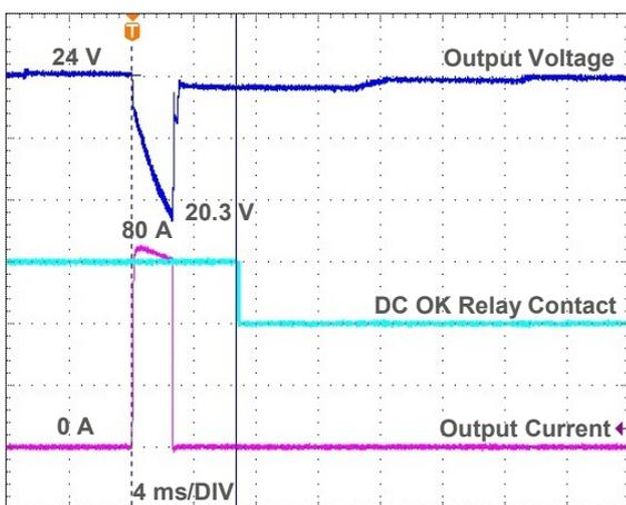
Fig. 8.3 APB 400% of nominal output current for 2 ms
