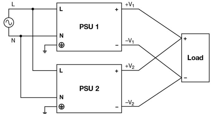
Fig. 9 Redundant & Parallel Operation Connection Diagram
