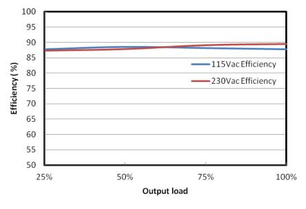
Fig.1 Efficiency versus output load
