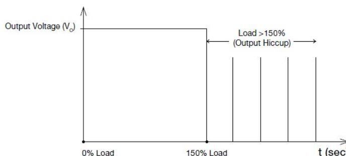
Additionally, if the  $I_o$  is  $< 115\%$  but  $> 100\%$  for a prolong period of time (depending on the load), the Over Temperature Protection (OTP) will be activated due to high temperature on critical components. The power supply will then go into hiccup mode until the fault is removed; and, the input voltage is removed, then reapplied.
