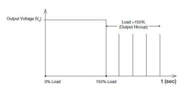
Additionally, if the I<sub>0</sub> is <115% but >100% for a prolong period of time (depending on the load), the Over Temperature Protection (OTP) will be activated due to high temperature on critical components. The power supply will then go into hiccup mode until the fault is removed; and, the input voltage is removed, then reapplied.
