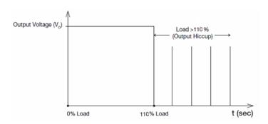
Additionally, if the lo is <110% but >100% for a prolong period of time (depending on the load), the Over Temperature Protection (OTP) will be activated due to high temperature on critical components. The power supply will then go into hiccup mode until the fault is removed; and, the input voltage is removed, then reapplied.
