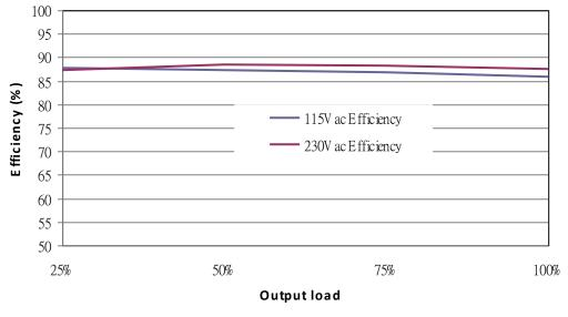
Fig. 1 Efficiency versus output load
