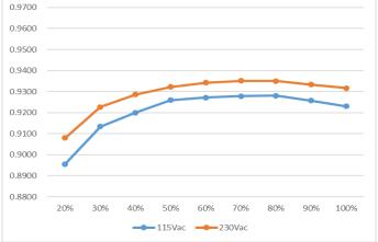
50% **─**115Vac **─**230Vac Figure 2. Typical efficiency Curve for MEU-650A24T
