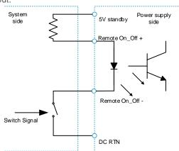
Figure 10. Remote On\_Off Connection
