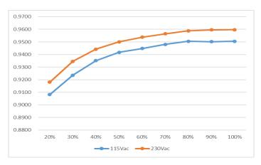
Figure 3. Typical efficiency Curve for MEU-650A48T
