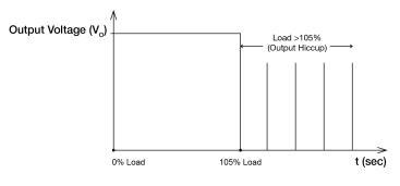
Additionally, if the I<sub>o</sub> is <105% but >100% for a prolong period of time (depending on the load), the Over Temperature Protection (OTP) will be activated due to high temperature on critical components. The power supply will then go into latch mode until the fault is removed and the mains is reapplied.
