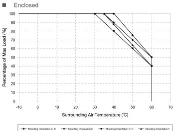
Fig.1.2 De-rating for Mounting Orientation A, B > 40°C de-rate power by 2.5% / °C De-rating for Mounting Orientation C > 35°C de-rate power by 2% / °C De-rating for Mounting Orientation D, E > 30°C de-rate power by 2% / °C De-rating for Mounting Orientation F > 35°C de-rate power by 2.4% / °C
