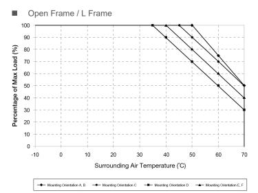
Fig.1.1 De-rating for Mounting Orientation A, B > 50°C de-rate power by 2.5% / °C De-rating for Mounting Orientation C > 45°C de-rate power by 2% / °C De-rating for Mounting Orientation D > 35°C de-rate power by 2% / °C De-rating for Mounting Orientation E, F > 40°C de-rate power by 2% / °C
