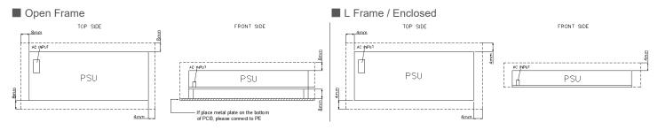
For safety reasons, please ensure the mounted device is kept safety distance as below at all sides from other components and equipments.
