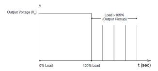
Additionally, if the Io is <105% but >100% for a prolong period of time (depending on the load), the Over Temperature Protection (OTP) will be activated due to high temperature on critical components. The power supply will then go into latch mode until the fault is removed and the mains is reapplied.
