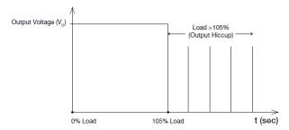
Additionally, if the  $I_{\rm O}$  is <105% but >100% for a prolong period of time (depending on the load), the Over Temperature Protection (OTP) will be activated due to high temperature on critical components. The power supply will then go into latch mode until the fault is removed and the mains is reapplied.
