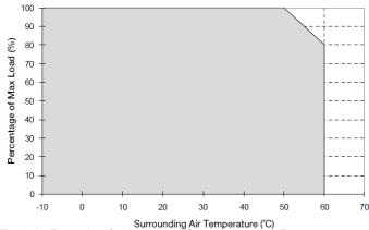
Fig.1.4 De-rating for Mounting Orientation A to F
