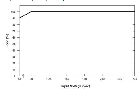
■ No output power de-rating for the input voltage range from 90 Vac to 264 Vac
