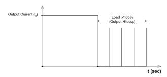
It is not recommended to prolong the duration of  $I_0$  when it is <105% but >100%, since it may cause damage to the PSU.
