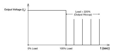
It is not recommended to prolong the duration of I<sub>O</sub> when it is <220% but >100%, since it may cause damage to the PSU.
