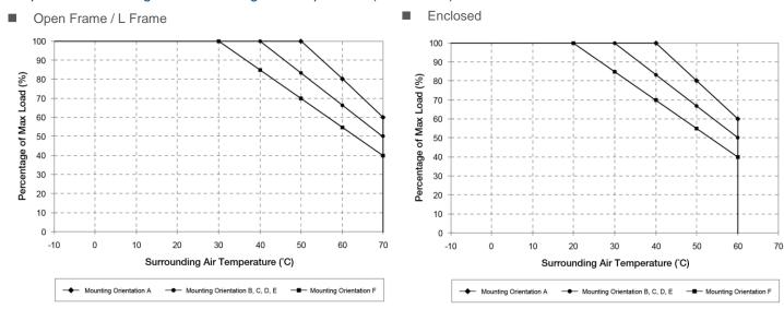
Fig.1.1 De-rating for Mounting Orientation A
