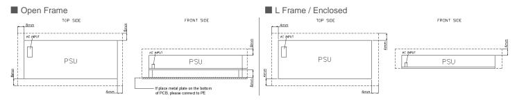
For safety reasons, please ensure the mounted device is kept safety distance as below at all sides from other components and equipments.
