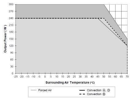
Fig. 1 De-rating for All Recommended Mounting Orientation
