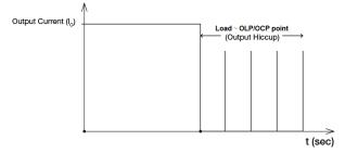
It is not recommended to prolong the duration of  $I_0$  when it is less than OLP/OCP point, but greater than 100%, since it may cause damage to the PSU.
