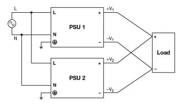
Fig. 4 Parallel Operation Connection Diagram
