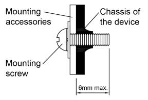
Only use M3 screw ≤ 6 mm (0.24 inch) through the base mounting holes. This is to keep a safety distance between the screw and internal components.
