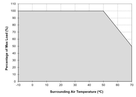
Fig. 1De-rating for Vertical and Horizontal Mounting Orientation<br/>> 50°C de-rate power by 2.5% / °C
