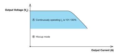
It is not recommended to prolong the duration of  $I_0$  when it is <101~130% but >100%, since it may cause damage to the PSU.
