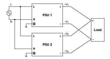
Fig. 4 Parallel Operation Connection Diagram
