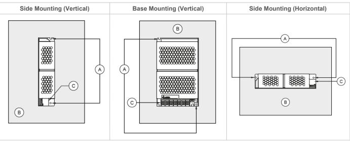
Fig. 2 Mounting Orientation
