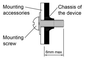
Only use M3 screw ≤ 6mm (0.23 inch) through the base mounting holes. This is to keep a safety distance between the screw and internal components.
