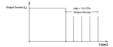
It is not recommended to prolong the duration of Io when it is <110% but >100%, since it may cause damage to the PSU.
