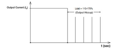
It is not recommended to prolong the duration of lo when it is < 110% but > 100%, since it may cause damage to the PSU.
