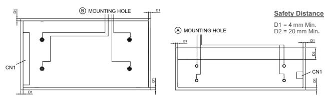
Fig. 3 Mounting Hole Locations and the Safety Distance
