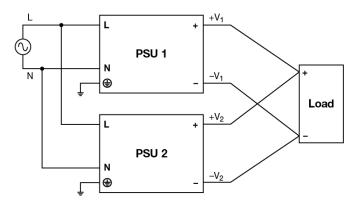
Fig. 6 Parallel Operation Connection Diagram
