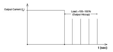
It is not recommended to prolong the duration of  $I_0$  when it is  $105\%\sim150\%$ , since it may cause damage to the PSU.
