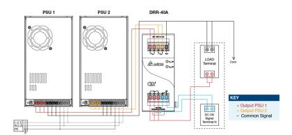
Fig. 5 Redundant Operation Connection Diagram
