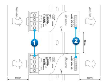
Note: 1. Input / Output terminal 2. Signals terminal
