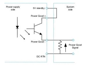
Fig. 23: Power good signal connection
