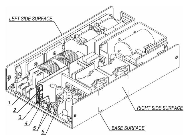
Fig.1: Components of the MEU-600C series
