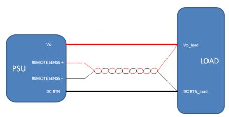
Fig. 25: Remote sense connection
