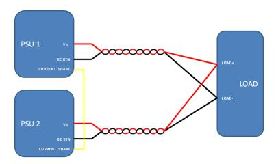
Fig. 27: Parallel connection without remote sense
