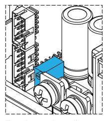
Fig. 7: Output voltage adjustment potentiometer
