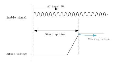
Fig. 17: Start-up timing sequence
