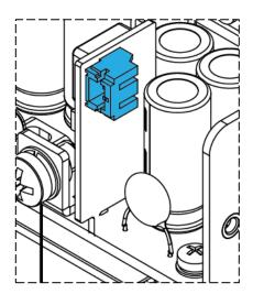
Fig. 9: 12V DC Output Connector (CN801)
