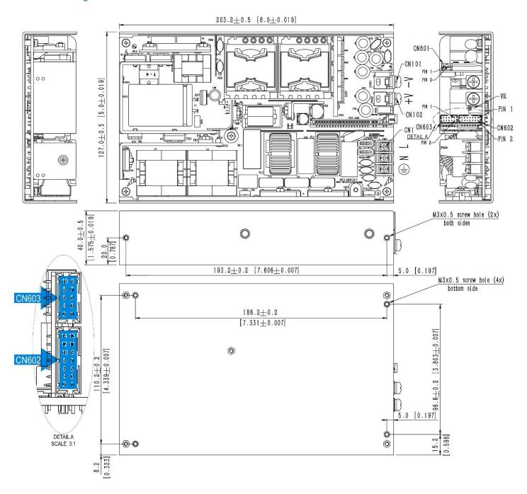
Fig. 16: Dimensional drawing MEU-600C
