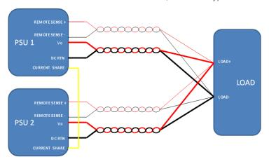
Fig. 26: Parallel connection with remote sense
