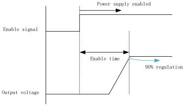
Fig. 18: Enable timing sequence
