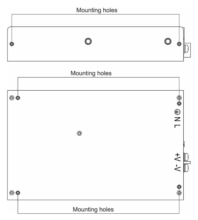
Fig. 15: Position of mounting holes
