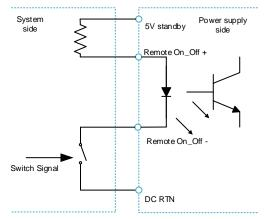
Fig. 22: Remote On\_off connection
