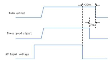
Fig. 24: Power good signal sequence
