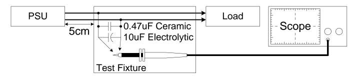
Fig. 3 Ripple & Noise measurement circuit
