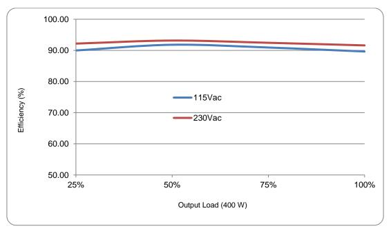
Fig. 1 Efficiency versus output load
