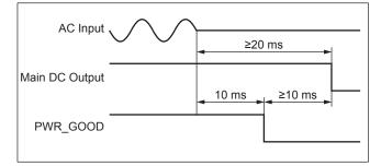
Fig. 13: PWR\_GOOD (Power Good) - Signal sequence
