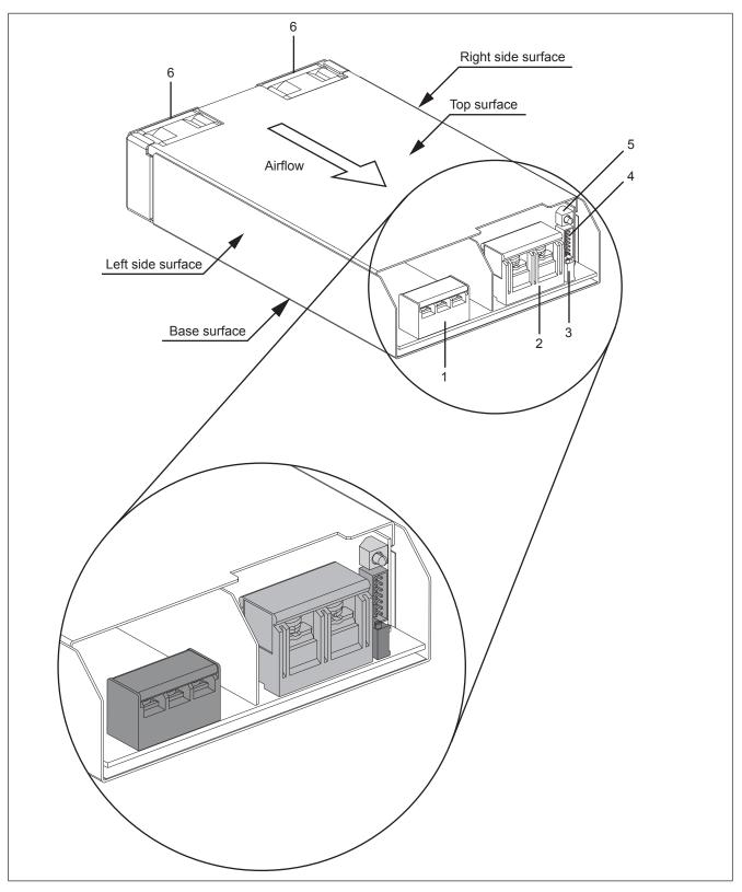
Fig. 1: Components of the IMA-x1000
