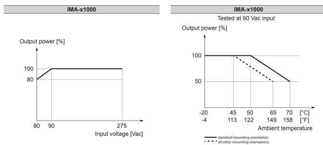
Fig. 26: Output power versus input voltage
