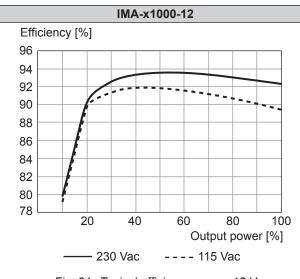
Fig. 31: Typical efficiency curves 12 V
