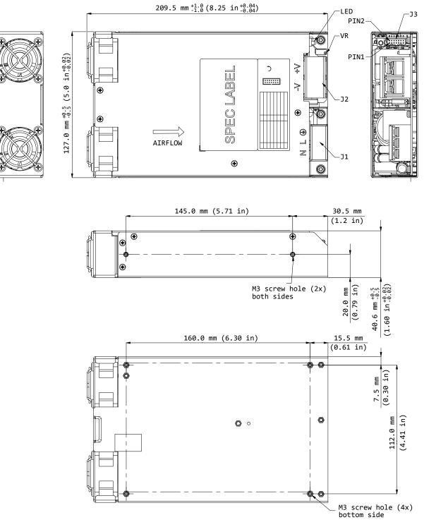
Fig. 25: Dimensional drawing IMA-x1000
