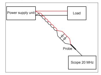
Fig. 14: Ripple measurement setup
