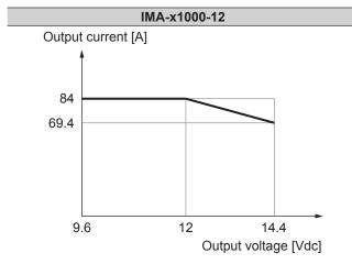
Fig. 28: Output current versus output voltage 12 V
