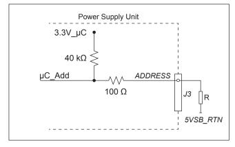
Fig. 16: Connecting resistor for I<sup>2</sup>C slave address
