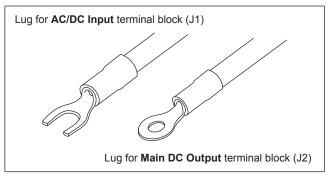
Fig. 17: Preparing cables for connecting
