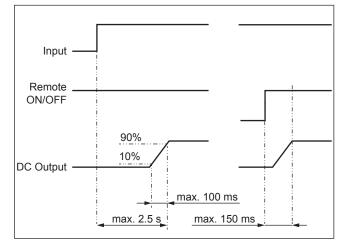
Fig. 8: Start-up timing YYPLI-Model
