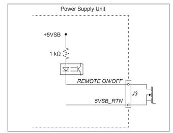
Fig. 11: Remote ON/OFF circuit diagram
