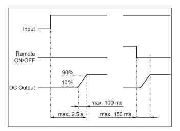
Fig. 9: Start-up timing YYPLY-Model
