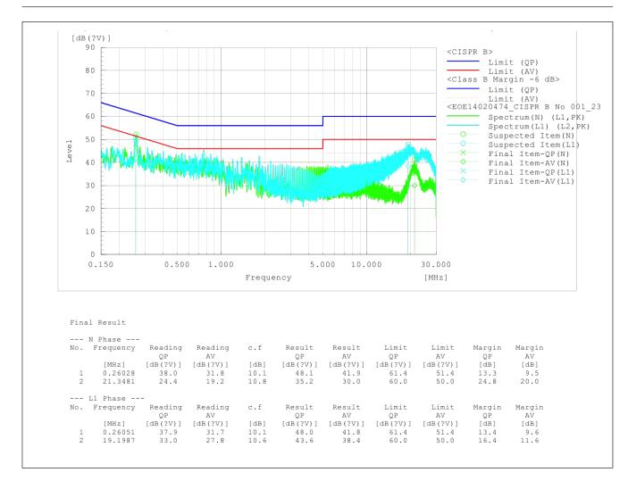
Fig. 18: Electromagnetic compatibility
