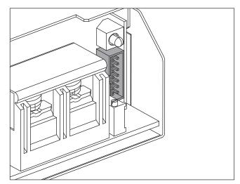
Fig. 3: Signal port and Auxiliary DC Output (J3)
