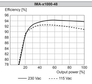
Fig. 32: Typical efficiency curves 48 V
