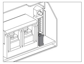
Fig. 6: Output voltage adjustment potentiometer
