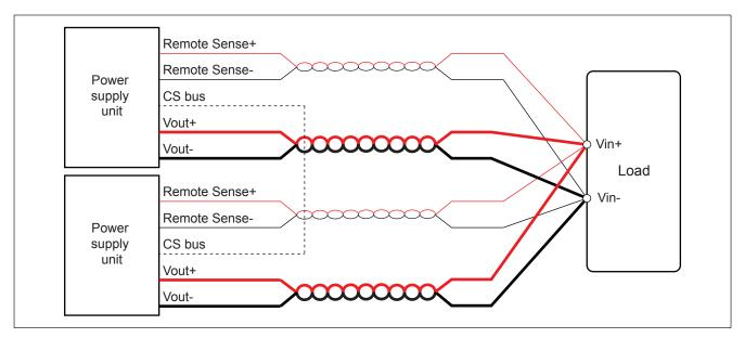
Fig. 15: Active Current Sharing (CS) bus - functional diagram
