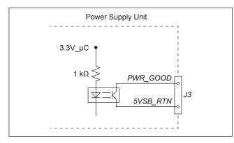
Fig. 12: PWR\_GOOD (Power Good) - Circuit diagram
