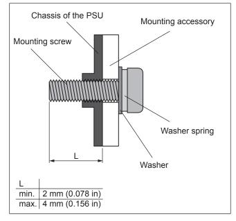
Fig. 19: Mounting the Power Supply Unit
