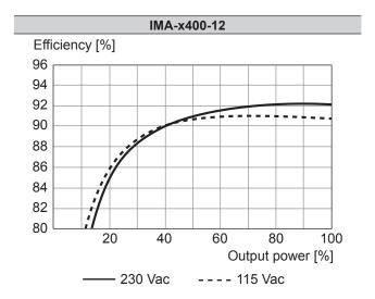
Fig. 37: Typical efficiency curves 12 V
