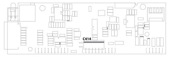
Fig. 12: Vertical conductor board; position of capacitors
