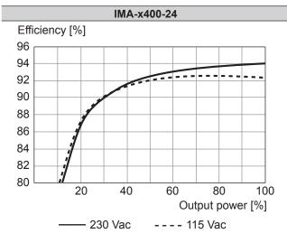
Fig. 38: Typical efficiency curves 24 V
