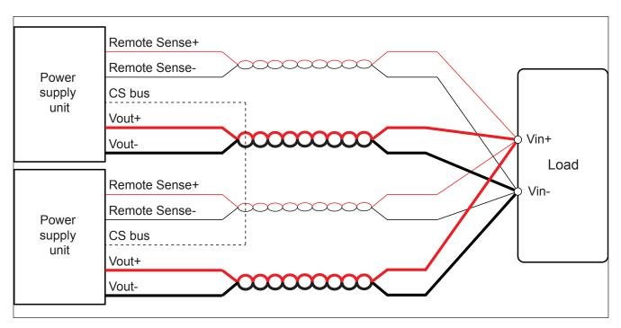
Fig. 17: Active Current Sharing (CS) bus - functional diagram
