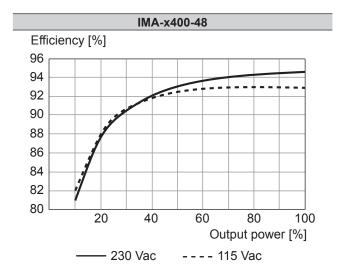
Fig. 39: Typical efficiency curves 48 V
