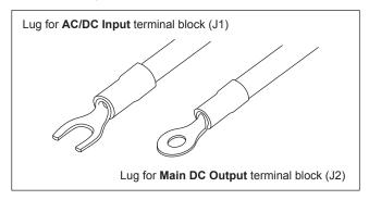
Fig. 19: Preparing cables for connecting
