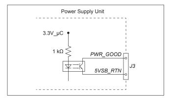
Fig. 14: PWR\_GOOD (Power Good) - Circuit diagram
