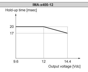
Fig. 34: Hold-up time versus output voltage 12 V
