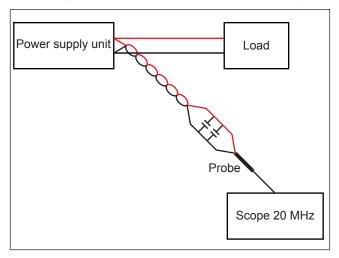
Fig. 16: Ripple measurement setup
