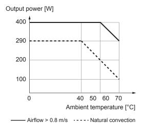
Fig. 28: Output power versus ambient temperature 12 V
