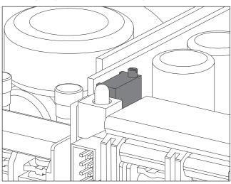
Fig. 6: Output voltage adjustment potentiometer
