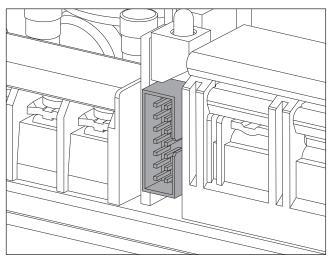
Fig. 3: Signal port and Auxiliary DC Output (J3)
