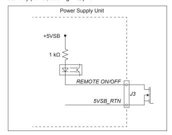
Fig. 13: Remote ON/OFF circuit diagram
