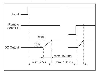
Fig. 8: Start-up timing ZYPLI-Model
