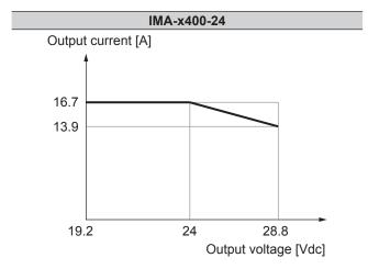
Fig. 32: Output current versus output voltage 24 V
