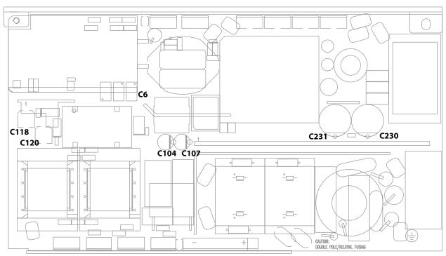
Fig. 11: Main conductor board; position of capacitors
