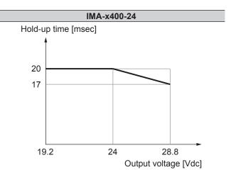
Fig. 35: Hold-up time versus output voltage 24 V
