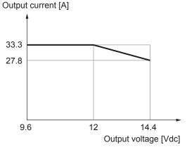
Fig. 31: Output current versus output voltage 12 V
