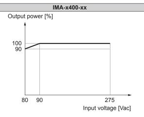
Fig. 30: Output power versus input voltage
