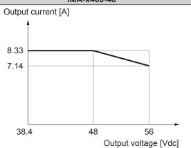
Fig. 33: Output current versus output voltage 48 V
