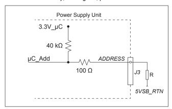
Fig. 18: Connecting resistor for I<sup>2</sup>C slave address
