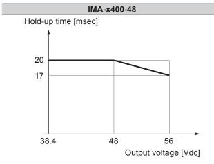
Fig. 36: Hold-up time versus output voltage 48 V
