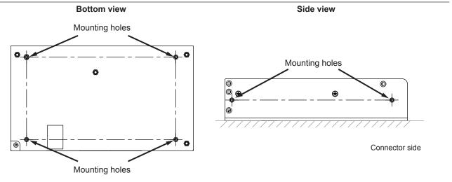
Fig. 26: Position of the mounting holes
