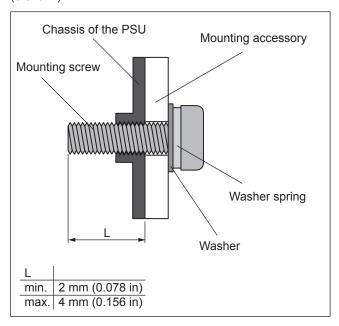
Fig. 21: Mounting the Power Supply Unit
