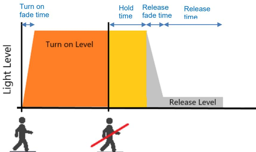
If the presence sensor detects movement at any point of Corridor mode sequence, the light level will revert to the Turn on level and go on as usual. All parameter are programmable using software GUI to fit application requirements.
