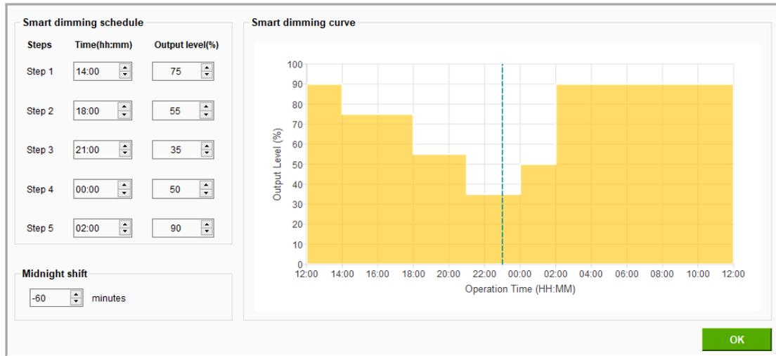
**Ratio Rescale Timer:** This mode is similar to Midnight Centric Timer that records the power-on time based on the local night time. The Ratio Rescale Timer software rescale programmed output power profile of each step by a calculated percentage of the recorded power-on time out of given 5 steps duration.
