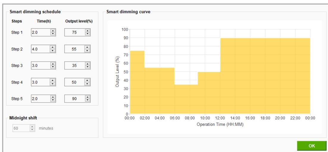
**Midnight Centric Timer:** This mode is a memory-based that automatically measures over the past two days the power-on time of the lighting installation at which is the naturally corresponded to night time. The Midnight Centric Timer software calculates the length of power on time and centralized from the given virtual midnight point and change the output level accordingly.
