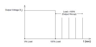
Additionally, if the I<sub>0</sub> is <130% but >110% for a prolong period of time (depending on the load), the Over Temperature Protection (OTP) will be activated due to high temperature on critical components. The power supply will then go into hiccup mode until the fault is removed; and, the input voltage is removed, then reapplied.
