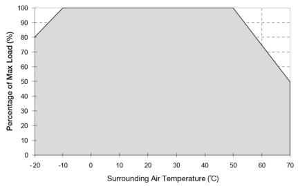
Fig. 1 De-rating for Vertical and Horizontal Mounting Orientation < -10°C de-rate power by 2.0% / °C > 50°C de-rate power by 2.5% / °C
