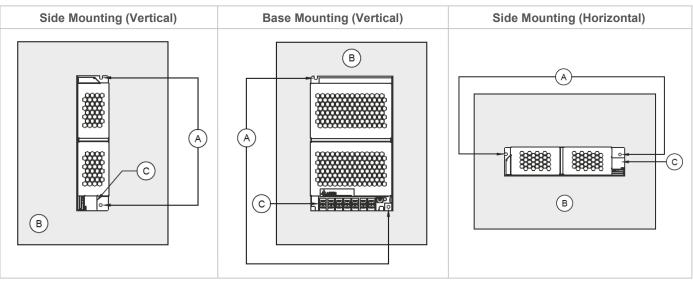
Fig. 2 Mounting Orientation
