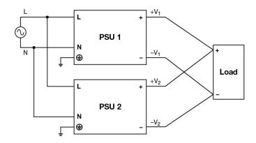
Fig. 4 Parallel Operation Connection Diagram
