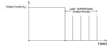
It is not recommended to prolong the duration of  $I_0$  when it is less than OLP/OCP point, but greater than 100%, since it may cause damage to the PSU.
