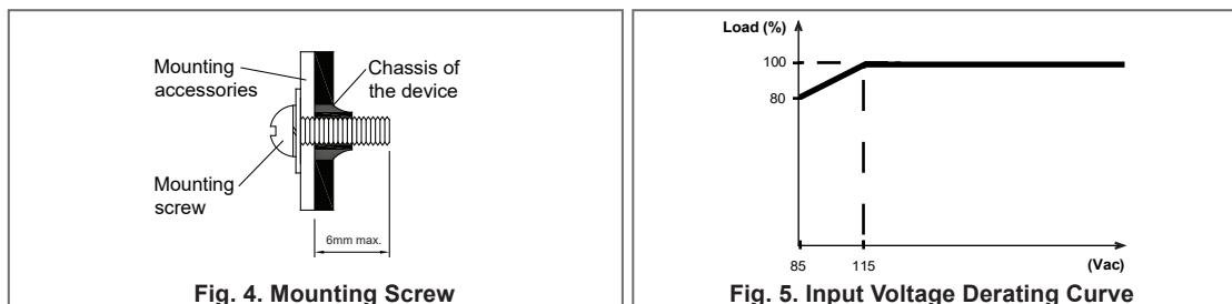
Fig. 4. Mounting Screw
