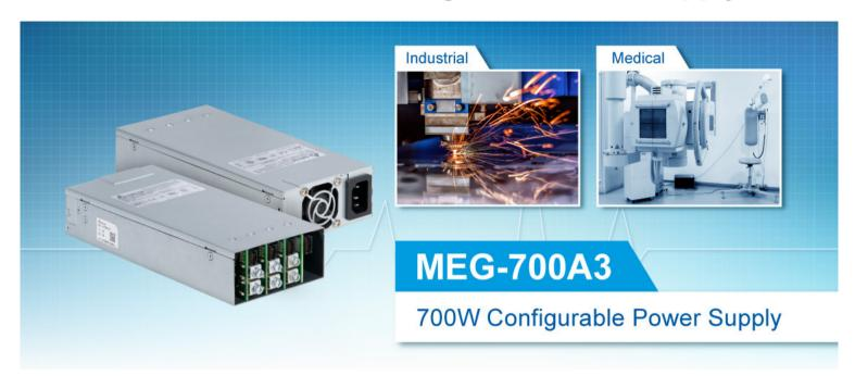
Delta Electronics's newest 700W MEG-A configurable power supply series is now available! The MEG-700A3 comes with 3 slots in compact size power density of 14.5W/in³ and efficiency up to 93%. The 3 individual modules allows a maximum output of 180W, 300W and 700W respectively. The output voltage can be configured between 2-60V with up to 6 different outputs. Additional features include current sharing, and intelligent fan speed control.
